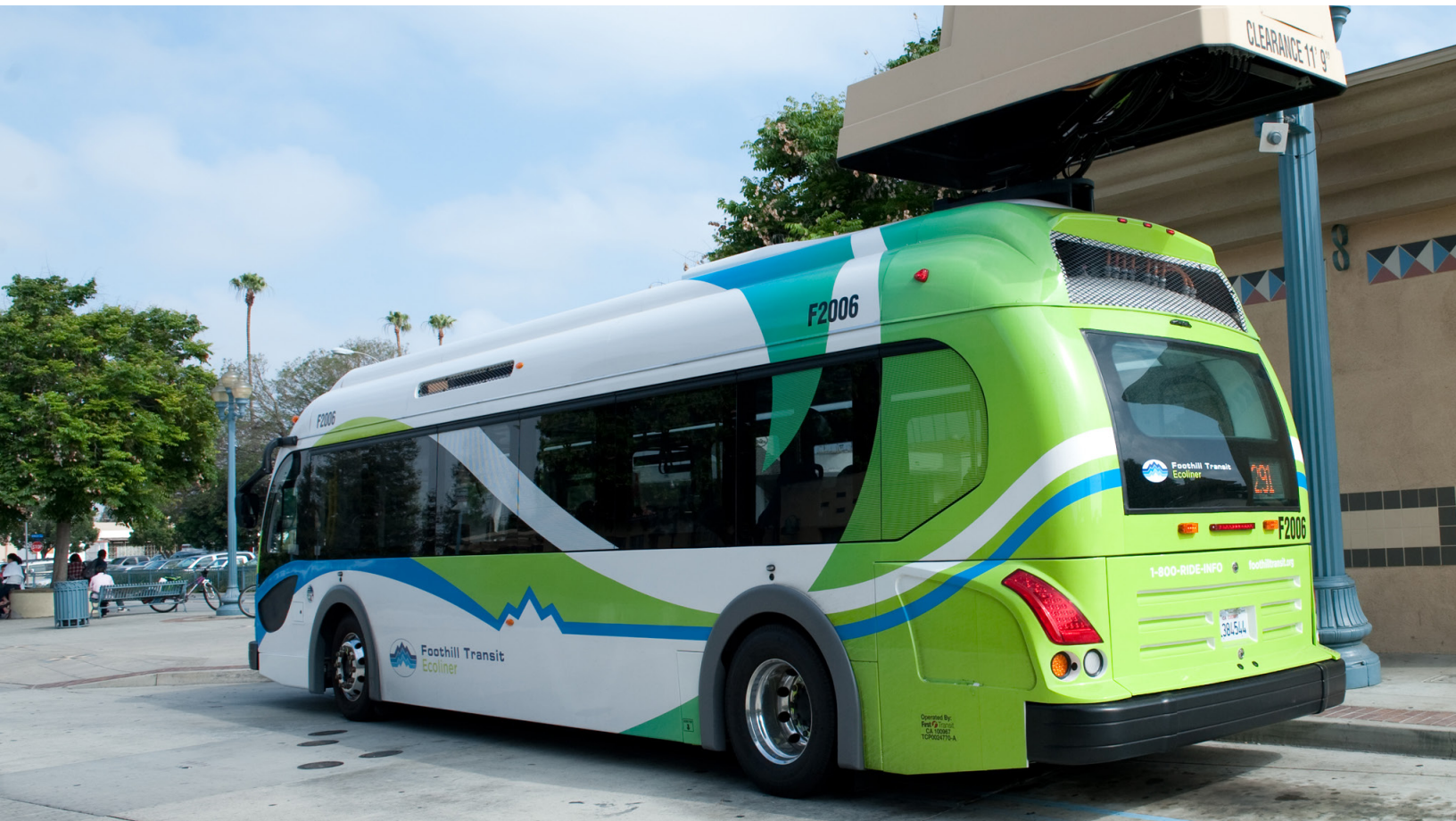
An all-electric transit bus parks beneath a rapid charging unit at the Pomona Transit Center. The bus, operated by Foothill Transit, recharges in 10 minutes thanks to specially designed fast charging lithium titanate batteries.
